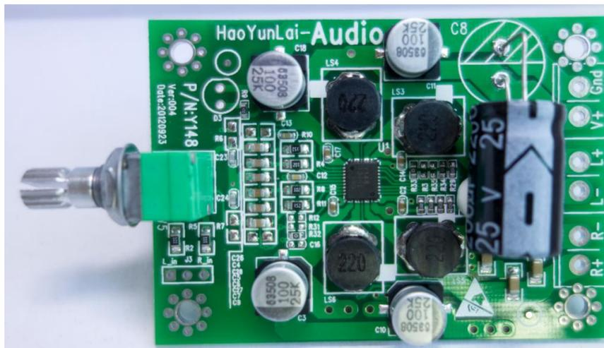
Figura: Amplifier board with YAMAHA YAD148 power amplifier
