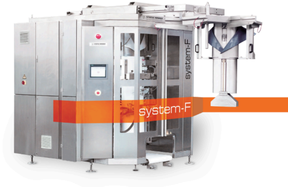
Figura 36: Envasadora System-F (“Proveedor: Statec-Binder”).
