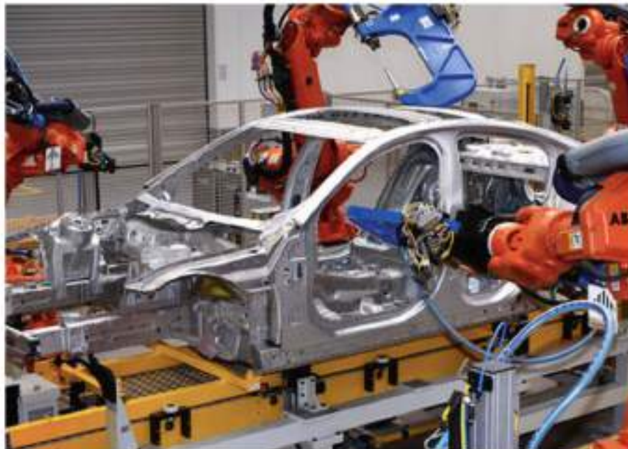
Fig. 4.2 Aluminium integral body shell during manufacture. Reproduced with kind permission of Jaguar Land Rover © Jaguar Land Rover Ltd
