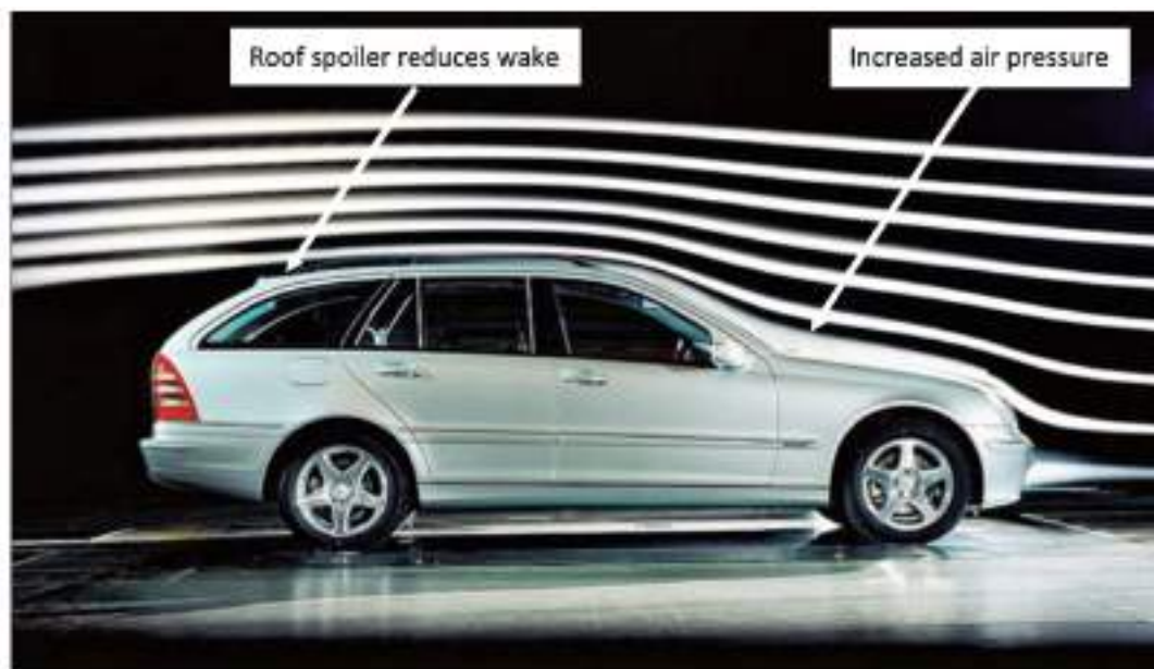
Fig. 1.4 Visualisation of streamlines in a wind tunnel test. Ref: http://images.gerrelt.nl/roofspoiler/mercedes_windtunnel_test.jpg
