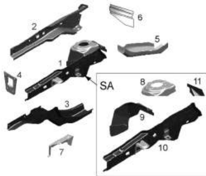
Fig. 4.5. Split scheme of front rail assy; in SA view, the set of rail boxing assy.
