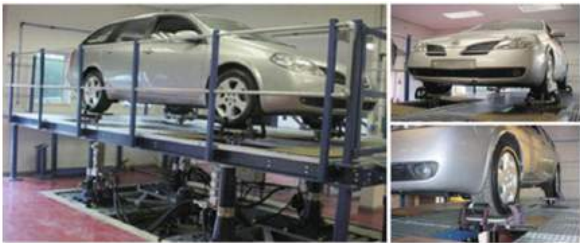
Fig. 4.26 Four poster dynamic test rig
