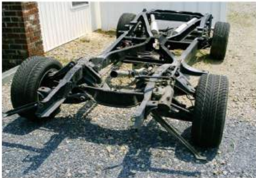
Fig. 4.1 Typical small truck chassis. Photo Christopher Ziemnowicz, licensed under [CC BY-SA 2.5], via Wikimedia Commons from "Wikimedia Commons"
