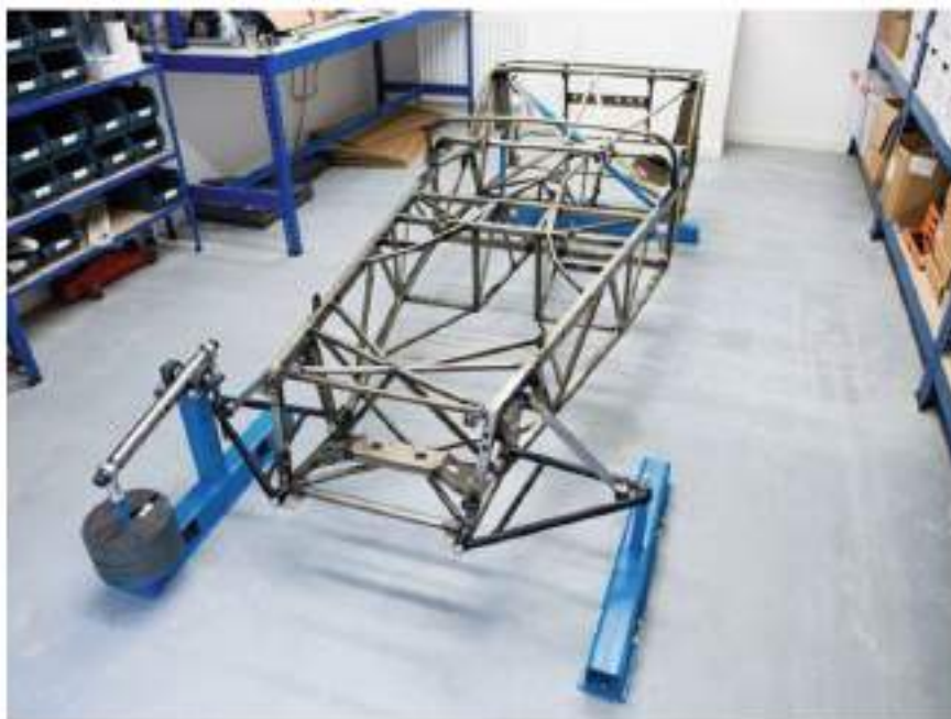
Fig. 4.7 Torsional test of space-frame chassis. Reproduced with kind permission of Simpack Engineering © Simpack Engineering Ltd.
