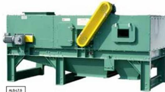
The high-energy permanent magnet inside a high speed drum creates a strong electromagnetic induction phenomenon on the surface of the drum. When the aluminum, copper, brass and magnesium (high conductive materials) pass through this magnetic field, the eddy current occurs repelling them respective to their conductivity thereby pushing each the distance determined by Fleming's left hand law creating separate piles for each type of material.
